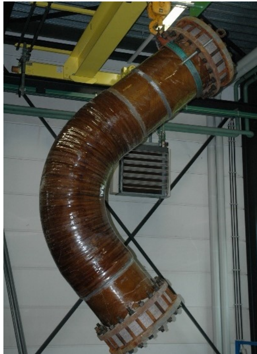
"1000 hrs test of Elbow and adhesive bonded joint acc. ASTM D 1598"
