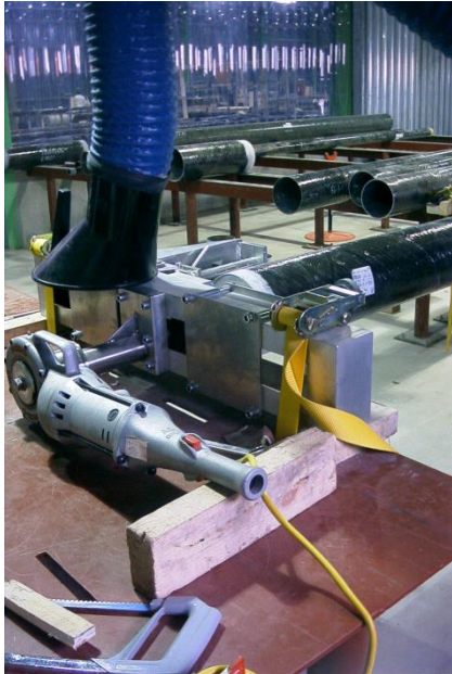
M87 shaving tool rigged up
