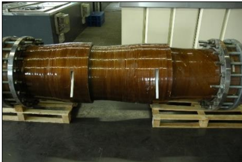
Figure 7: Bonded GRP spool (Courtesy Fiberdur Germany).
