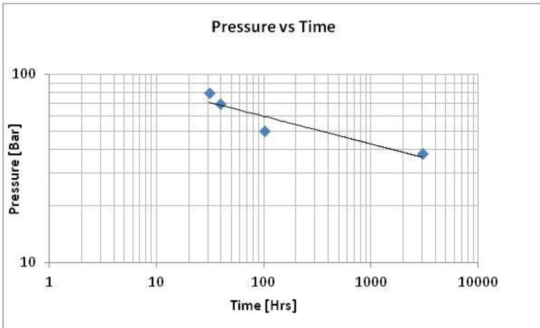
Figure 9. Regression curve for TPR Fiberdur pipe example.
