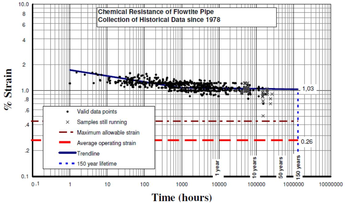
Figure 1. Test results: 30 years of regression testing (Courtesy: Flowtite, Amiantit Group, Norway).
