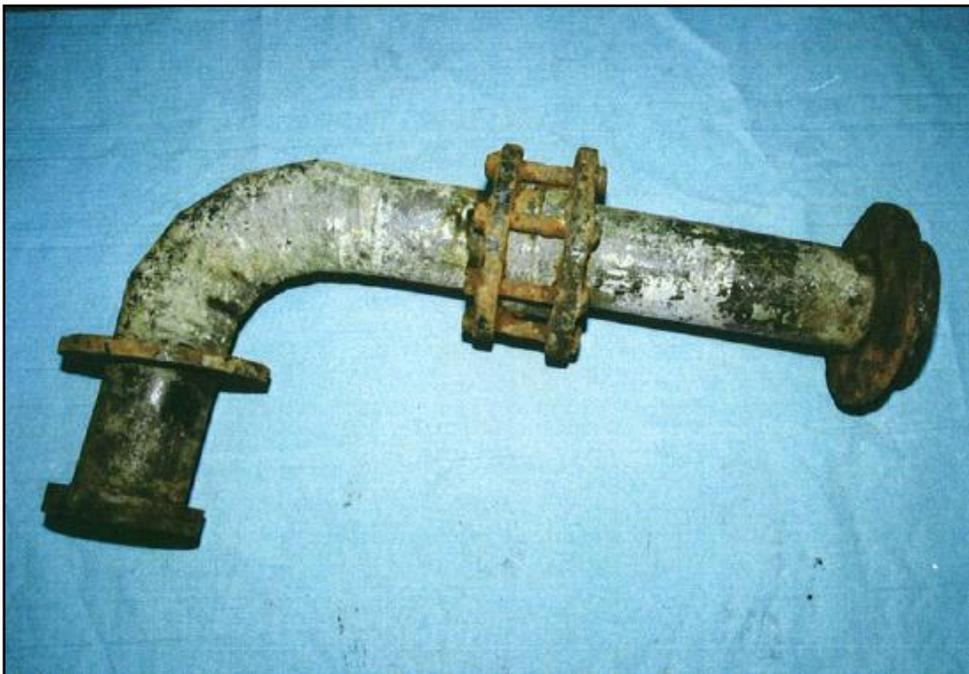
**Figure 8. 25 year old pipe test sample. (Courtesy TPR Fiberdur, Germany)**
