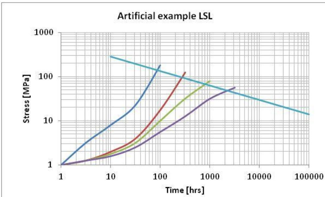
Figure 10. Low speed loading tests intercepting regression line.
