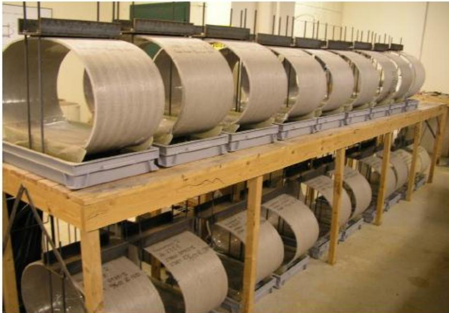
Figure 2. Overview test samples (Courtesy: Flowtite, Amiantit Group, Norway).
