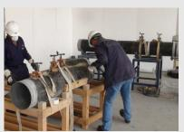
checked the spools and joints for deviating dimensions based on ISO 14692. Subsequently, the spools designed for 16 bar were subjected to a hydrotest at a pressure of 40 bar for 1 hour.
